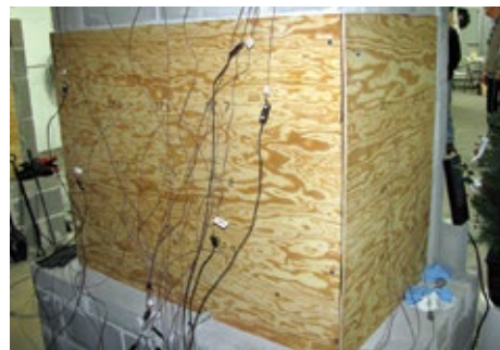
Thermocouples attached to test fireplace in Wardenclyffe Hearth Lab.
