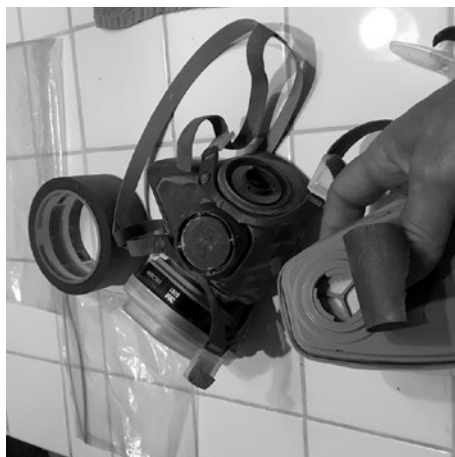
Cover the connection point of the filter after use to keep out contaminants.
