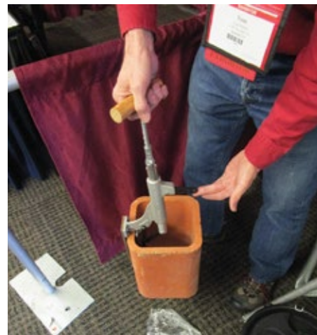
Tom Martin of A.W. Perkins demonstrates use of the PterodacTILE tile remover/setter tool.
