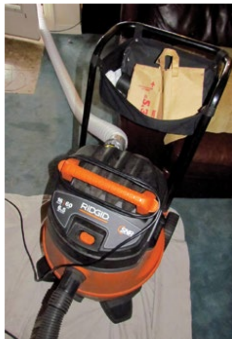
Ridgid vac modified with two HEPA filters and vented to the outside.
